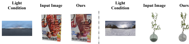
Figure 15. Failure Cases. Left: High-frequency details (e.g., text) are blurred due to voxel resolution constraints and VAE compression loss. Right: Transparent objects exhibit checkerboard artifacts. While 3DGS theoretically supports alpha blending, data scarcity in current datasets leads to inaccurate density estimation for refractive surfaces.
