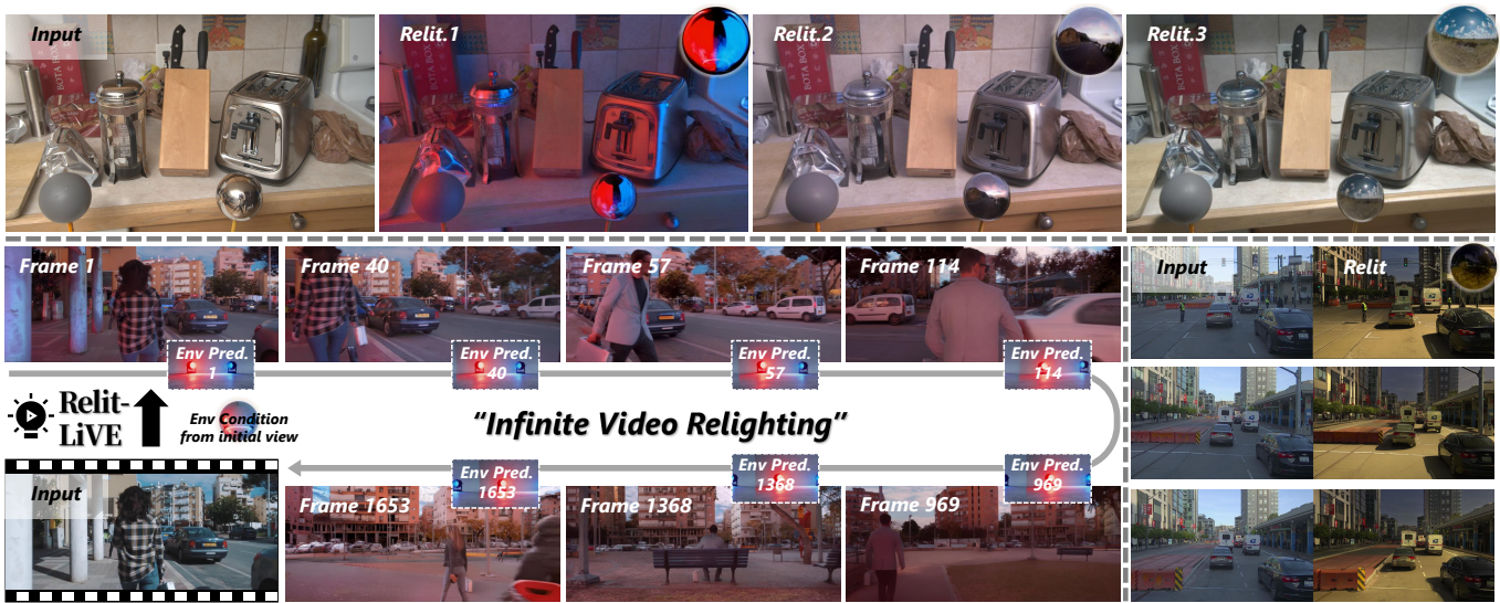
Fig. 1. We present RELIT-LIVE , a novel video relighting framework that produces physically consistent and temporally stable results without needing prior knowledge of camera pose. This is achieved by jointly generating relighting videos and environment videos. Additionally, by integrating real-world lighting effects with intrinsic constraints, the relighting videos demonstrate remarkable physical plausibility, showcasing realistic reflections and shadows.
